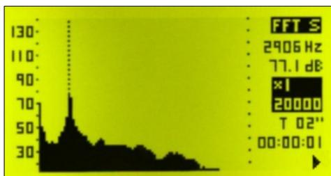
The extended frequency module of the **SC310** sound level meter adds 2 modes of measurement: Extended frequency module for 1/3 octave band analysis and FFT (Fast Fourier Transform) narrow band frequency analysis mode.
