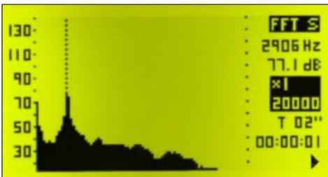
The module for vibration measurements of the **SC310** sound level meter adds 2 measurement modes; the human exposure to whole-body vibration in buildings mode and the FFT (Fast Fourier Transform) narrow band frequency analysis for vibration.
